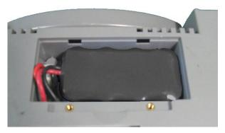
e) Shut the battery compartment cover and fix the screws.
