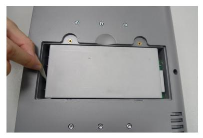
e) Shut the battery compartment cover and fix it with the screws.
