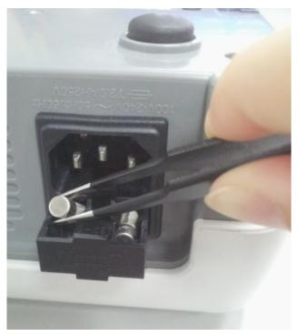
5) Push the fuse container all the way back in position.
