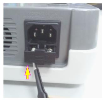
4) Take the fuse out and replace it with a new one that is supplied by the manufacturer or of the same specifications.
