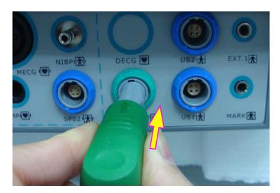
When disconnecting a transducer, pinch the afterbody of the transducer plug and pull it out slightly.
