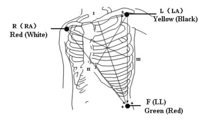
Figure 9-2 Placing 3-lead ECG Cable
