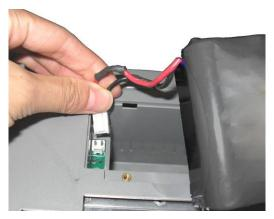
d) Put the battery and the cables into the battery compartment.
