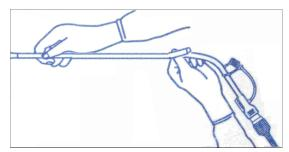
Figure 7-6 Separate the Introducer
