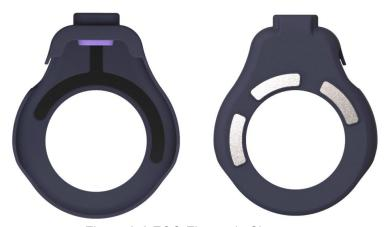
Figure 3-8 ECG Electrode Sleeve
