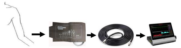
Figure 8-10 Connection for NIBP measurement
