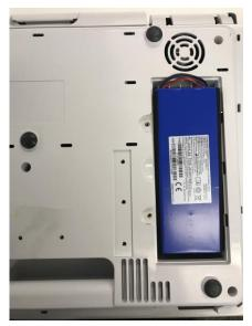
e) Shut the battery compartment cover and fix the screws.
