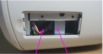
Battery Connecting Metal Insert Cable & Connector
