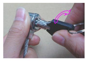
2 Insert the lock hook into security slot on the back of the main unit. Rotate the key anticlockwise to close the lock hook.
