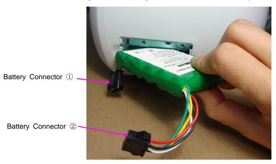
3 Keep pushing the battery into the compartment until the metal insert springs back to lock the battery.
