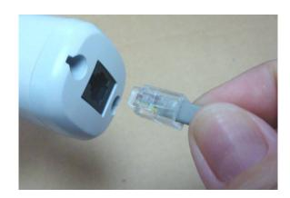
To disconnect the probe, press the housing of the modular plug and then pull it out.
