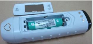
3 Close the battery compartment cover and fix it with the screw.
